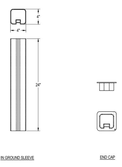
Sleeves shall be constructed of 6063-T6 extruded aluminum and require bury in an 8" x 30" minimum footing. Actual sleeve depth shall be 24" and be designed to allow removal of 4" square uprights on Bison in-ground soccer goals. Sleeve shall have a removable steel top cap. Installation to be completed in accordance to manufacturer's instructions. Do not scale drawings. Weight approximately 5#/each.
