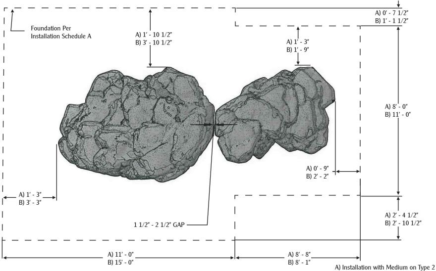
NOTE: Ensure that boulders are placed exactly as shown. No other arrangement or positioning is allowed.
