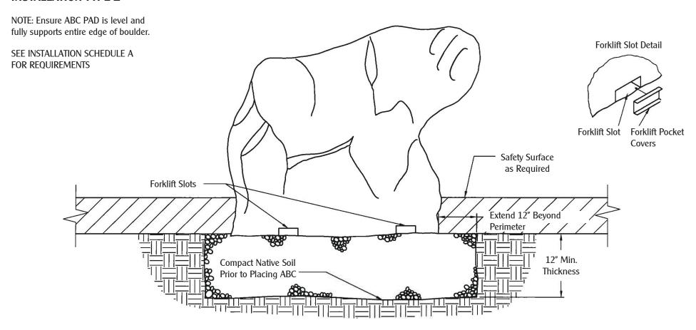
12" Thick Layer of Aggregate Base Course\* (ABC) Compacted to 98% (Standard Proctor)
