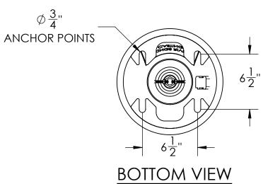
BASE: CONSTRUCTED OF DURABLE, CORROSION RESISTANT, HEAVY WALL CAST ALUMINUM.
