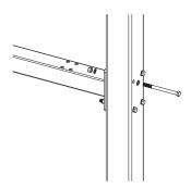
If building a Kolo shelter with Decker racks, lift the Decker Beam in place and fasten with (8) 5/8x7.5" bolts, lock washers and nuts.
