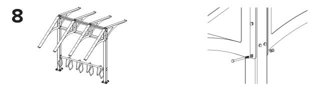
Fully secure the Rafters with (6) 5/8x7.5" bolts, (12) lock washers, and (6) nuts for each pair of Rafters
