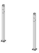
Place Uprights based on footing diagram and drill (4) 1/2" diameter pilot holes in concrete 13" deep for each Upright. Remove Upright and use pilot holes to drill 7/8" diameter holes 13" deep. Arrange special inspection of anchor holes and anchor/epoxy installation per IBC 2012. Consult Simpson Set 3G epoxy instructions for further detail. After inspection a sufficient epoxy cure time, the Uprights may be placed over the threaded rod and secured with washers and nuts finger-tight.
