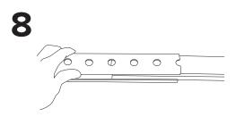
If splicing an additional length of track, slide the Splice Slotted Track over the last 6" of the 96" Slotted Track.
