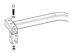
Fasten the Channel Supports to the uprights with  $\frac{1}{2}$ " x 3" bolts,  $\frac{1}{2}$ " washers,  $\frac{1}{2}$ " lock washers, and  $\frac{1}{2}$ " nuts.
