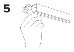
Insert the Trolleys into the open end of the 96" Slotted Track.
