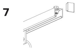
If no more Track Racks are going to be spliced together, apply hex head cap screw, washers, nut and End Cap in the open end of the Slotted Track to keep trolleys from sliding out.
