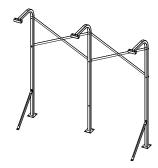
A) For single-sided units, attach Knee Braces to the first Upright and then every other Upright with 3/8" x 3" bolts, 3/8" washers, 3/8" lock washers, and 3/8" nuts. Anchor each Knee Brace by drilling a 3/8" hole and fastening with a wedge anchor.
