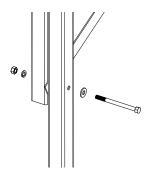
B) For double-sided units, fasten the Double-sided Uprights and Upright Braces to the Uprights with  $3/8" \times 3"$  bolts, 3/8" washers, 3/8" lock washers, and 3/8" nuts.
