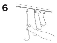
Insert the hooks through the holes in the tabs that are hanging down from the Trolleys. Each hook length should be at least 3" different than the neighboring hook.
