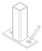
Place the rack in the desired location. Use a marker or pencil to outline the holes of the flange onto the base material.
