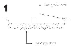
Place corrosion resistant sleeve (min. 4" inside diameter) in sand pour bed in exact location where rack will be installed. Make sure top of sleeve is at same level as desired finished concrete surface. Fill sleeve with sand to keep it in place and prevent it from filling with concrete.
