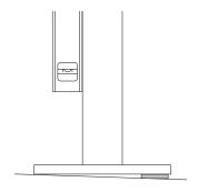
Place rack (and washers to level rack if necessary) over holes.
