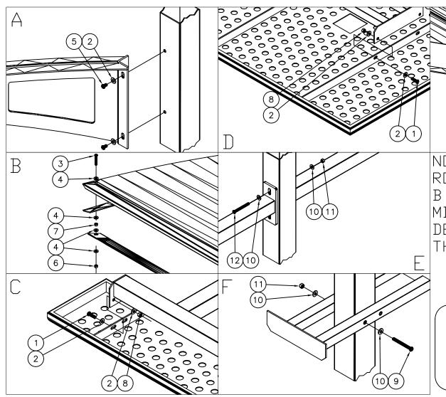
NOTE: WHEN ATTACHING ROOF SECTIONS, DETAIL B IS USED ON THE MIDDLE AND END HOLES. DETAIL G IS USED ON THE OTHER 5 HOLES.
