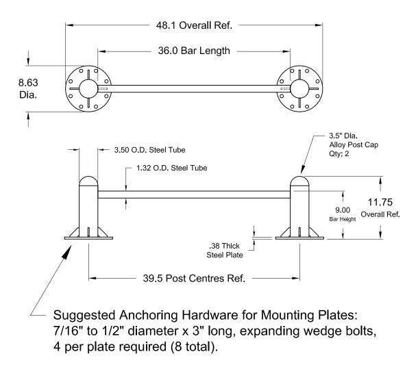
**Notes:** Use the fully assembled unit as a drill template.
