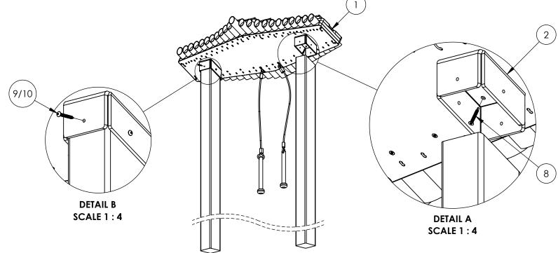
Step 1: Excavate two 10" diameter holes, 36" deep, and 32" on center at the installation location. Contractor can modify Post to desired height. Post Length = Frost Depth (36" Recommended) + Finished Post Height
