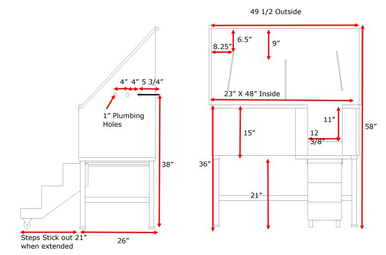
Available as Left, Right or center drain.  $3.5^{\prime\prime}$  drain hole, located  $7^{\prime\prime}$  on center from the left or right.
