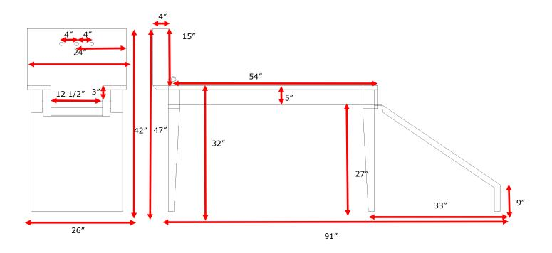
Available as Left, Right or center drain. 3.5" drain hole, located 7" on center from the back wall.
