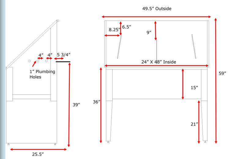
Available as Left, Right or center drain. 3.5" drain hole, located 7" on center from the left or right. (12" from front of tub and 12" from the back of the tub)
