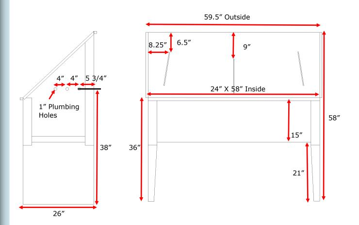
Available as Left, Right or center drain. 3.5" drain hole, located 7" on center from the left or right.
