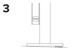
Place rack (and washers to level rack if necessary) over holes.
