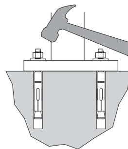
Thread nuts onto anchors, leaving approximately 1/4" of the anchor protruding, and tap into surface. Tighten nuts down to secure rack.
