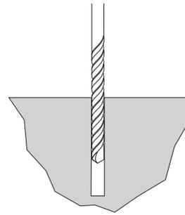
Drill 3/8" diameter holes 3" deep into surface. Make sure the holes are at least 3" away from any cracks in the base material.
