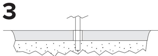
After appropriate cure time, dig out sand from sleeves and insert racks, making sure they are level and at the appropriate height. Pour in Por-Rok or epoxy grout and allow to set.
