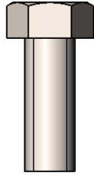
3/8" x 1" Machine Bolt
